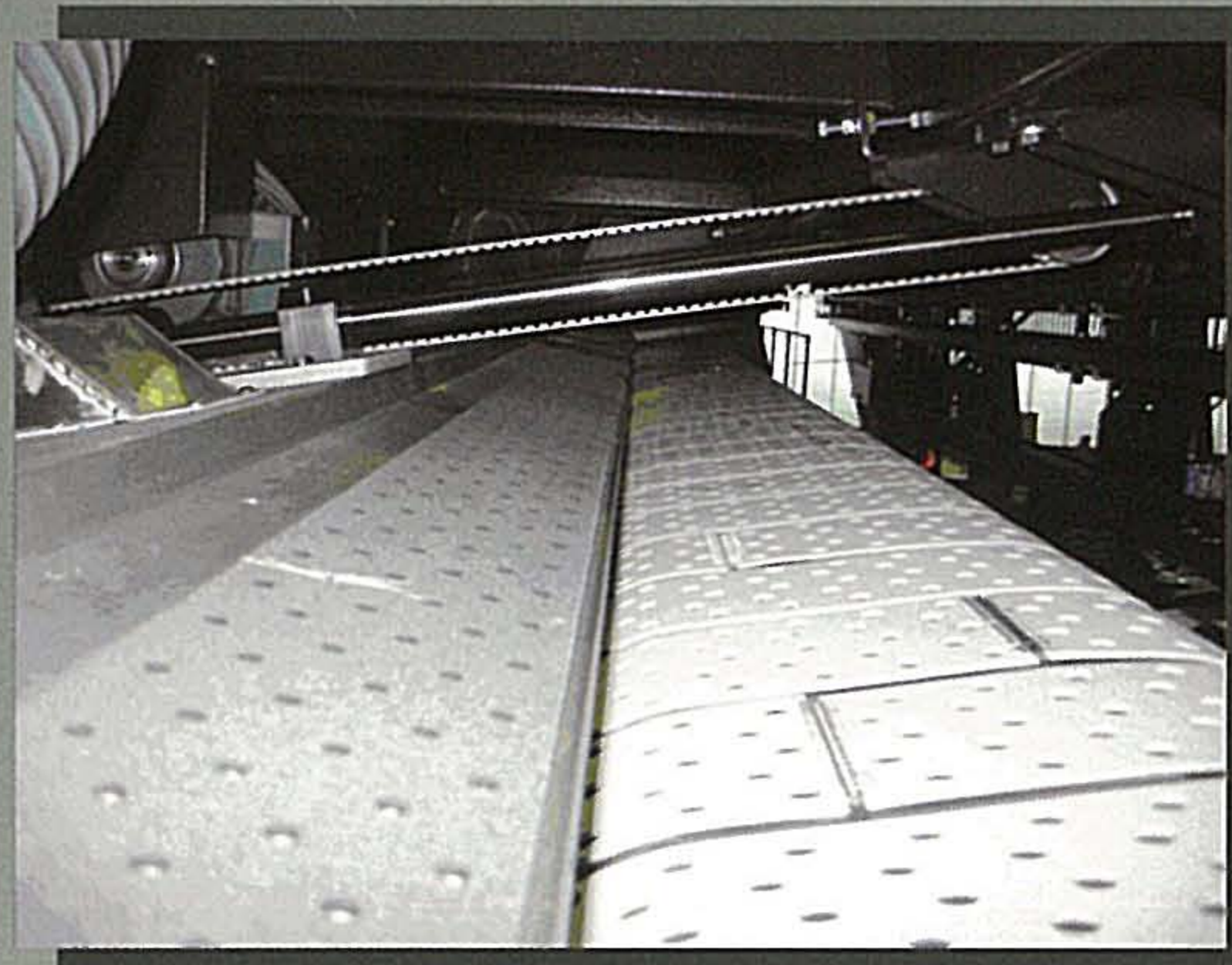
Feeding beam with high vacuum and vacuum under transport belts to secure quality lay down. Maintenance free beam guiding.
