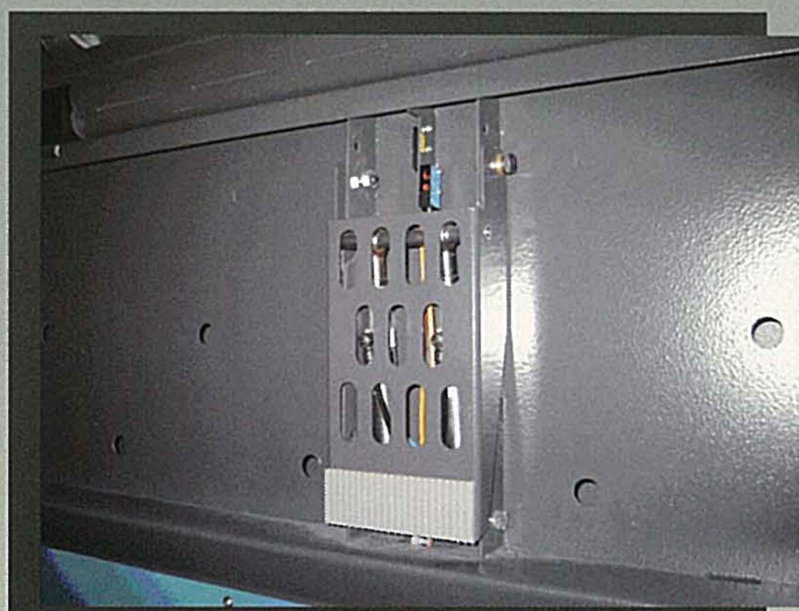
Lifting system to get a straight leading edge for heavy big sheets.
